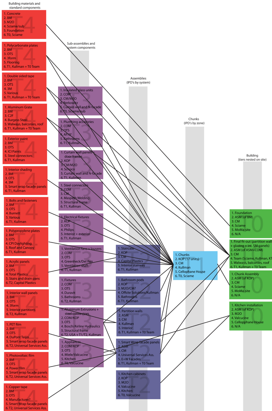
Figure 2. System structure model of the Cellophane House™. Each coloured box is a separate delivery. Lines illustrates integration or nesting into other deliveries while the different tiers are expressed as T4 to T0
